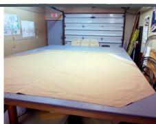
Here is our aft cover all stapled and ready to be brought over to the sewing table to get sewn and bound. We heat the edge with a hot knife to prevent fraying. Stitch just in from the folded edge on all sides and stay-stitch the outside edge of the aft cover. Stitch down all selvage edges where reinforcing strips are joined. We prefer to run over all stitching rather than use a lot of back tacking on all covers like these.
