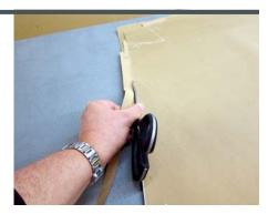
With scissors, we trim away the extra reinforcing fabric even with the edge of the aft cover. We will not make the corner cutout at this time, but will leave the corner squared off. Using a long-arm stapler, reach in and staple around the cutout close to the edge. We will cut the corner out after we stay-stitch the edge in a later step.
