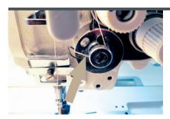
When sewing with any machine and there is a sound different from the usual chug, chug—stop! The arrow in the photo points to a problem with the thread path. Always look for the simple solution first. Check the thread path to be sure it is clear, and then change the needle. According to Ron at Groz-Beckert, changing the needle is a very inexpensive fix that cures a multitude of problems.
