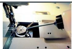
The arrow points to the groove in the bobbin case into which we place a drop of oil every other bobbin change. This is the fastest-moving part in the machine, and oiling here will increase the life of the hook. We also place a drop of oil on our finger and rub the needle bar at the same time to increase the life of the bar. This is in addition to regular routine machine oiling.
