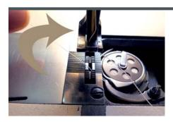
This is a trick that ace sewing-machine mechanic Freddie from Sloan Machinery taught us. Pull out the bottom thread and at the same time move it in a circle around the feed dog opening following the arrow. If there is a burr in that area, the thread will break and you know where to look.
