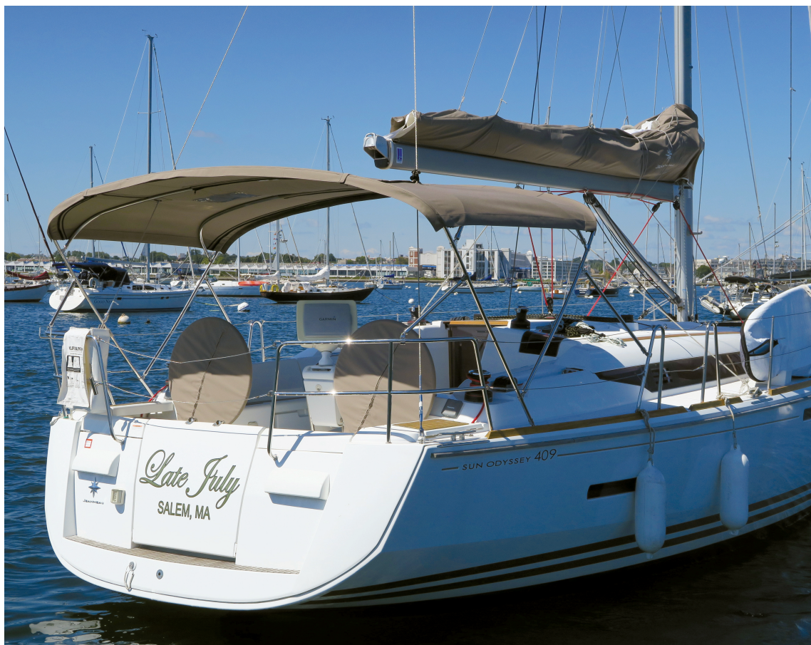
This Jeanneau 409 is moored in historic Salem Harbor in Massachusetts. The bimini features dual backstay cutouts to extend sun coverage aft over the helms.
