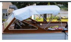
Now, after marking the forward edge of the bow from the underside, we release our pattern from the double-sided tape and re-stick. We want our pattern to be smooth between the mid bow and the aft bow. These steps are performed on each side of the boat after initially securing our pattern blank along the center line of the frame and windshield.
