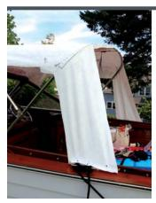
We added another layer of double-sided sticky tape on top of our pattern and stick on a square of pattern material to make our sport top tails. Be sure it lays in smooth and fits the contours of the frame. Now mark the cut line on the aft bow.
