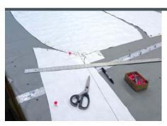
Back at the shop, we have started working up our pattern. This is the aft end where the top and tails meet. Notice the darts at the mid bow and the tails for proper fit. We have rounded the inside connection between the top section and the tail. This adds a touch of styling and if we were to add side curtains, this would enable the attachment zipper to round the corner.
