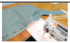
We have top-stitched the aft end. Be sure the aft bow pocket is out as shown in the photo. Also notice that the tail and visor are connected as one piece.
