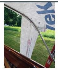
This is a view from the underside showing the overlap of the tail pattern pieces. Notice the strapping tape at the hold-down strap position inside the tail, so it is hidden. The strapping tape is holding the upward force of our frame preload down the center line of our frame. It is important that the strapping tape is placed at the exact spot that our strap will be when our sport top is completed for proper preload and fit.
