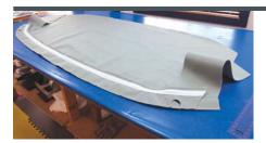
Here the aft end is assembled and stapled in the proper stacking order prior to stitching.
