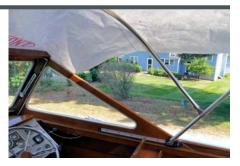
This is a view from the underside. Notice the marker line from when we fitted the forward section. We now have to draw another line after fitting the aft section. These lines merge near the center of the frame creating a dart of excess material to be removed in later steps.
