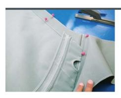
This is the end of the aft pocket, cut up to allow a zipper to pass. We have pinned out the side to remove any waviness prior to stapling the aft pocket down as this is important to the final fit. Notice the cutout for our hold down strap just inside the wing. This is in the exact spot that we had out strapping tape while patterning.
