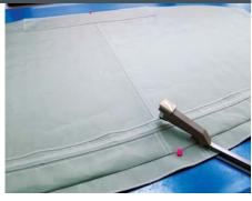
The bow pocket is flipped to the underside. Notice we have pinned out the center seam prior to stapling the pocket down. Failure to do this with any top will result in a non-even pull and will cause wrinkles when installed.
