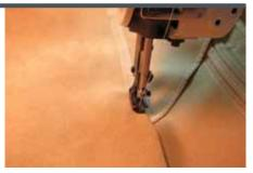
We are topstitching the entire aft seam of the dodger. In the photo we are about to topstitch over the interconnection between the pocket and the wing. Be sure that the aft pocket in this step faces out under the wing.
