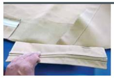
Here is a peak under the lid. Notice that the wing is stapled down first with the pocket on top. Notice that our aft pocket is in three sections with a gap between them. This is so our aft welded handle can pass through and be zipped onto the aft frame.
