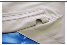
We have flipped the dodger to the backside and turned the pocket to the inside. The aft pocket has been stitched down through the top football panel and leather chafe below it. No need to ease off the ends of the aft pocket becasue it extends far enough down the side of the dodger not to be a problem. Notice that the wings extend out from the middle of the seam between the top football panel and the aft pocket.
