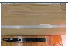
After topstitching, flip the assembly over and stitch down the forward pocket. It is important to ease off the ends of the forward pocket by ½ inch—only the center needs to be tight. We have mentioned this before in past articles, but it is so important to do this that it warrants repeating: If you were to stitch this forward pocket down flat along the straight line in the photo you would have diagonal ripples in your top panel.
