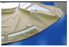
In this step we are joining the aft pocket and the wings in one seam. This is the area of concern for some fabricators. Notice the stacking order of the pieces. Also notice that the pocket extends inside the wing by about 6 inches on each side. This particular dodger has straps instead of bars aft so we have included cutouts just inside the wings to accommodate them
