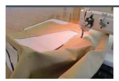
We are topstitching the seam between the top football panel and the forward panel assembly. The seam contains the forward pocket. Be sure when topstitching that the forward pocket faces out under the forward windows.
