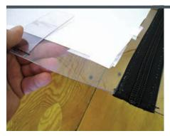
Split the zip on each side of the smile slightly and install a slider on each end to close the zipper. Now stay stitch the zipper and the top of the cover flap together at the very top and trim even with the glass. It should be noted that we use single-pull sliders only, as no one ever opens a smile from the outside.
