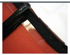
The cover flaps are now stapled with a long-arm stapler to the outside of the window vinyl. It must cover the zipper installed on the inside of the window vinyl. This is where the extra 2 inches at the top of each side of the cover flap is needed to account for any small adjustments in alignment.
