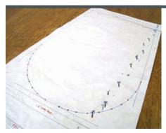
This is our pattern with the smile window marked on it with a Sharpie marker. We punch holes along the length of the smile so that we can transfer the center line marks of the smile to the window vinyl underneath. We also use the pattern to transfer the center line marks to the fabric used to make the cover flap.
