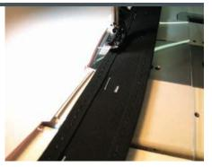
9 Starting at the top inside edge, stitch the cover flap on each smile. Stitch on the binding stitch line and remove the staples. Do not stitch the outside edge or your window will not open. In the case of a "frown" instead of a smile, stitch the cover flap on the outside edge and leave the inside edge unstitched.
