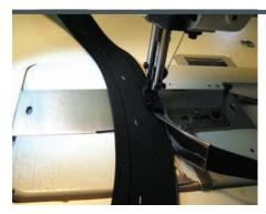
We now bind the inner and outer side of each cover flap with 3/4-inch binding. Keep in mind that this is a single-ply cover flap.
