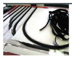
The stack of smile windows with zippers installed, and finished cover flaps ready to be installed.
