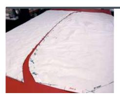
In this photo we have cut the side curtains off the pattern and cut the top mid seam apart on the pattern along the marking on the underside for the secondary bow. We transferred this line from the underside to the outside by using a rolling pounce wheel to make perforations. Notice that there are hash marks for seam and zipper alignment where the pattern pieces are separated.
