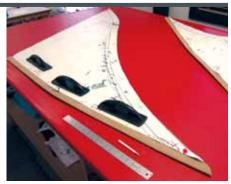
In this photo we have the side curtain patterns on top of the side curtains in order to transfer the hash marks for proper side curtain alignment with the Navy top. First we stitch the zips onto the Navy top and then we transfer the hash marks to the bottom of the zipper from the hash marks on the Navy top. Finally, we remove the bottom half of the zips and align and stitch them to the hash marks on the top of the side curtains.
