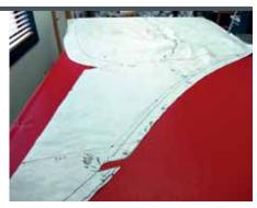
A close-up of one side curtain is shown here. We have punched holes where the fabric bottoms join the clear vinyl. This is done in two sections: the bottom piece and the piece that runs forward along the windshield. This facilitates fabrication in that no one joining piece is wider than the width of the fabric.
