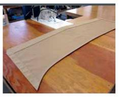
This photo shows the forward section of the Navy top with the sides folded in and the forward reinforcement in place, stapled and ready for stitching. We will add rubber spray welt and binding to the forward edge where the snaps will go.
