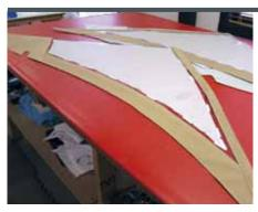
These are the almost-complete side curtains. We have used our large binder to finish the top edges. We need to add the aft sleeves that hold 1-inch flat battens to stiffen the aft edge from flapping while underway. We also need to bind the bottom edge, but first let's go over the fabrication of the aft sleeve.
