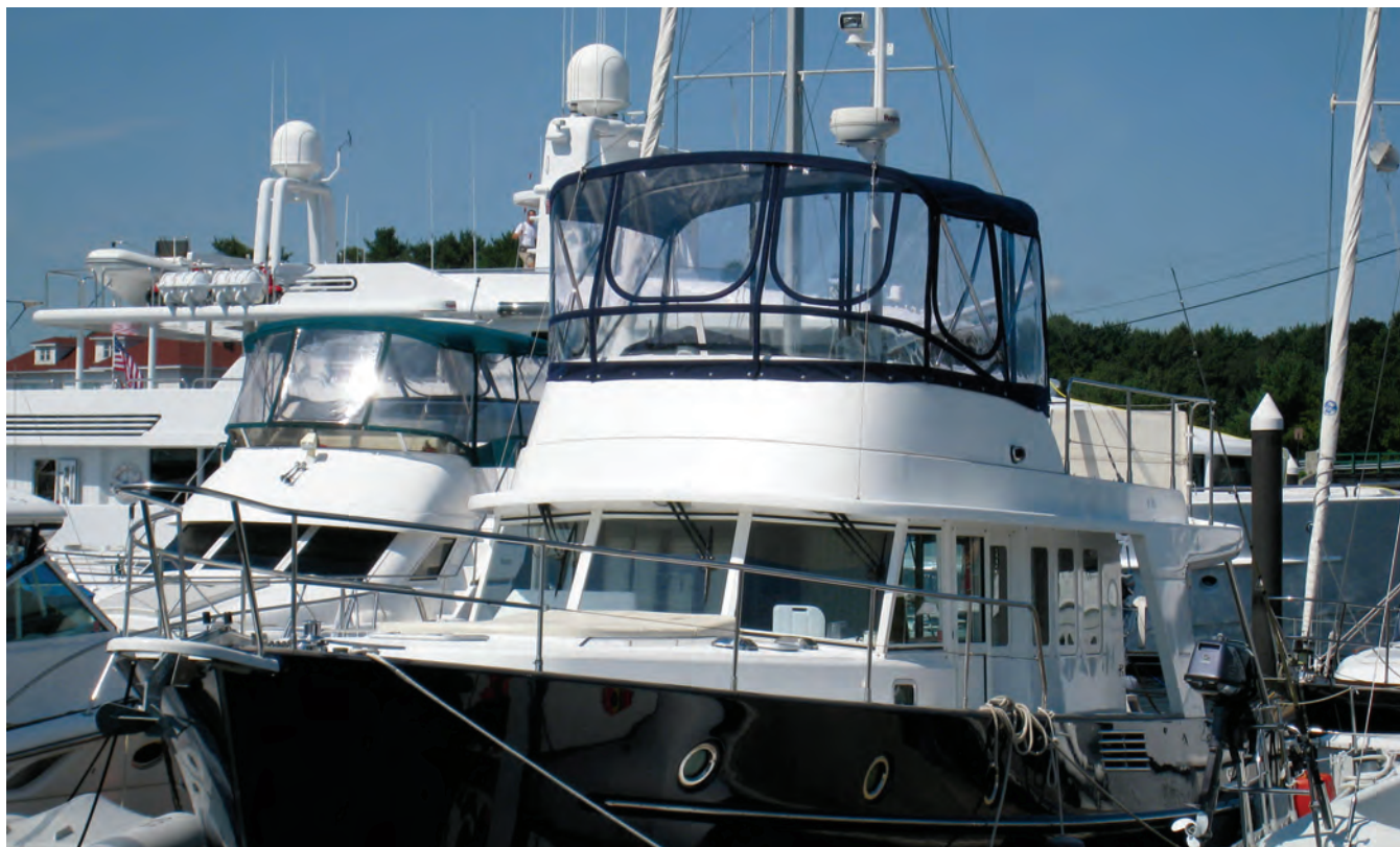
A A Hood bimini enclosure on a Beneteau Swift Trawler 42. The forward enclosure panels are tucked under the windshield to the fasteners with a seam hidden along the edge of the windshield by fabric strips.
